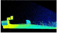
Fig. 3 Noisy data under fog haze weather condition
