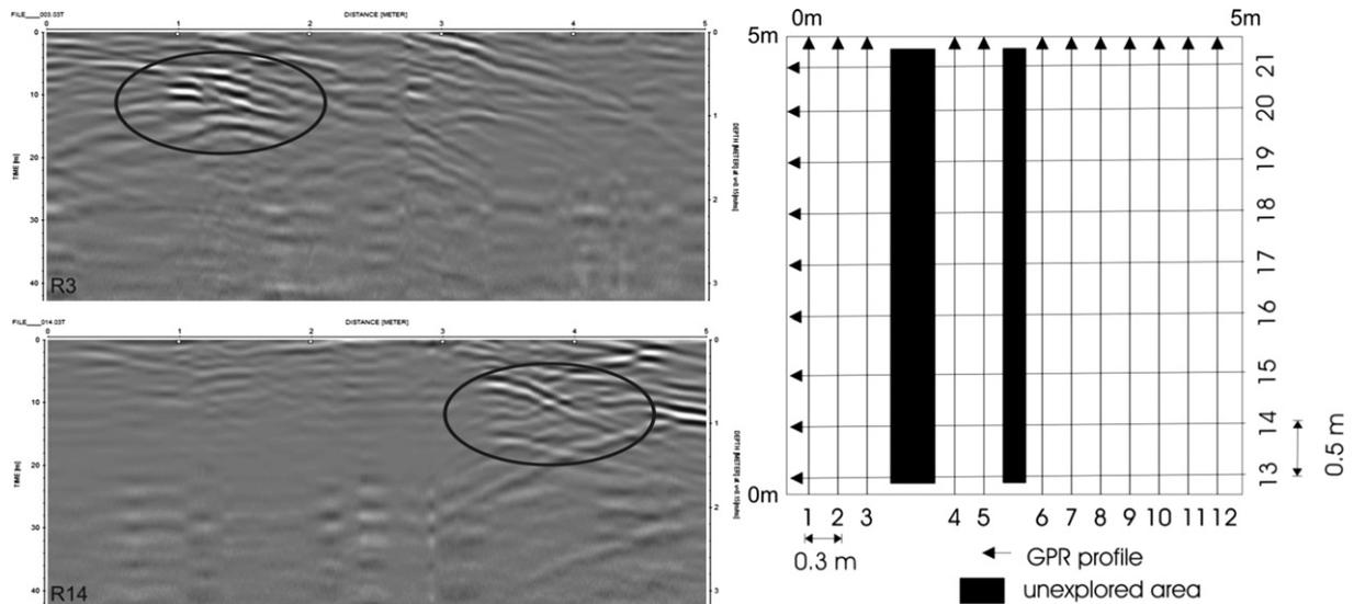
Fig. 7. Eastern side. Two GPR profiles (upper left and lower left) and grid of the investigated area (right). The black circles highlights the reflection zones.
