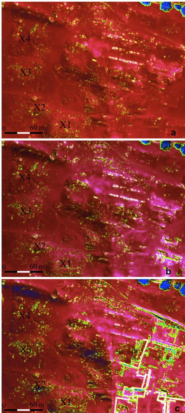
**Fig. 4.** RGB composition of Moran, Getis and Geary indices (R: Moran; G: Getis; B: Geary) applied to panchromatic images of 2002 QB (a), 2005 QB (b) and 2008 WW1 (c).
