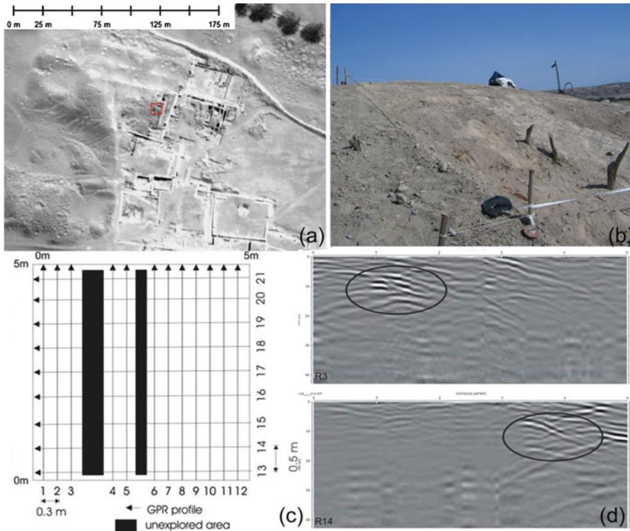
**Fig. 14.18** (a) Location of the area investigated by georadar method, indicated by a *red square box*; (b) detail of the investigated area; (c) georadar profiles performed on a 5 x 5 m area where geomagnetic technique provided high values of magnetic field; (d) migrated radargrams R3 and R14, where it is possible identify some superficial reflection hyperbolas (indicated by *black ellipses*)
