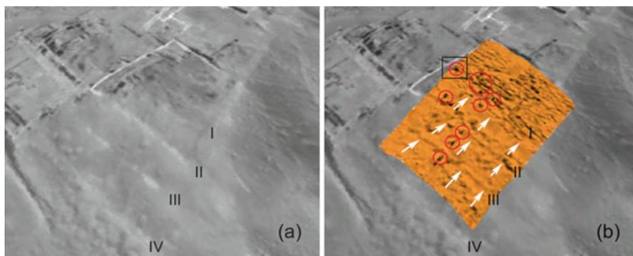
**Fig. 14.16** (a) 3d satellite image (2008 WV1) visualization of northern slope of *Piramide Naranja*, and (b) geomagnetic map overlaid on the satellite image. The *white arrows* denote linear magnetic signals, the *red circles* indicate more intense magnetic signals, the *black block* evidence the anomaly selected in collaboration with archaeologists to be firstly investigated by GPR and then excavated
