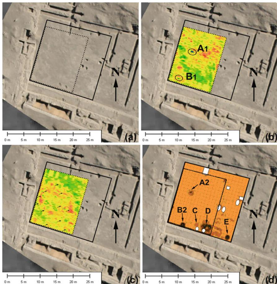
**Fig. 14.21** (a) The investigated area: the two rectangles with *dot* and *continuous* line indicate the areas investigated by georadar and geomagnetic method, respectively; (b–c) GPR time slices at 15 and 30 cm, respectively; (d) geomagnetic map
