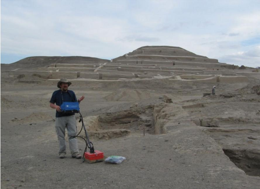
**Fig. 14.6** Georadar system
