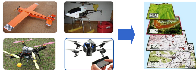
Fig. 3 Digital acquisition of archaeological sites with low-altitude unmanned remote sensing
