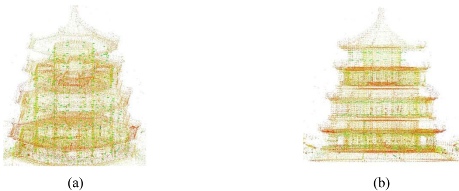
Figure 5. point clouds of cross-sections of the pillars in the whole tower (marked as green in the above figures). Figure (a) is the oblique view from above where the pillars are seen more clearly; Figure (b) is the view from the front where the cross-sections can be seen more clearly)
